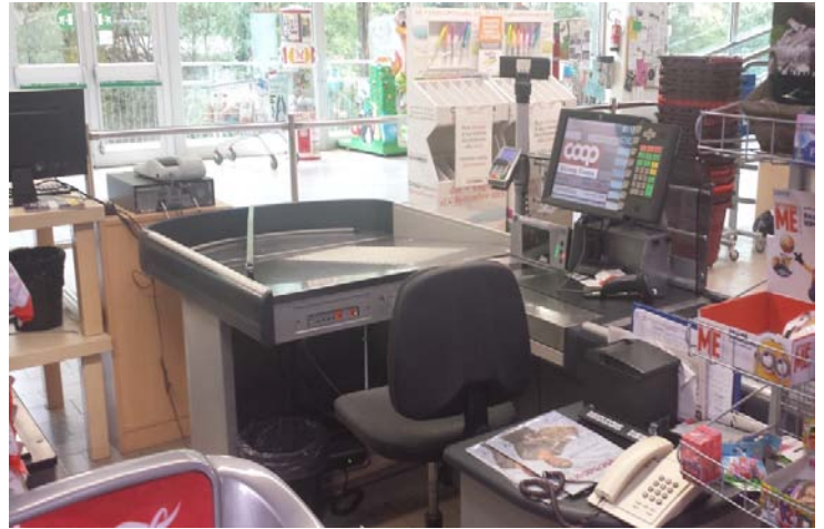
This European set-up includes a seat with a back, and room for the cashier's knees to fit under work surfaces.
